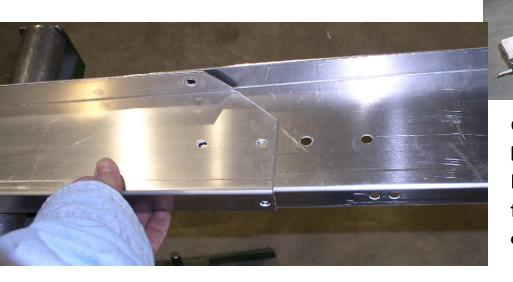
Connect the existing ramp beam to the 10' extension. Fasten with two 1/4: bolts and flange nuts fasten on the top only.
