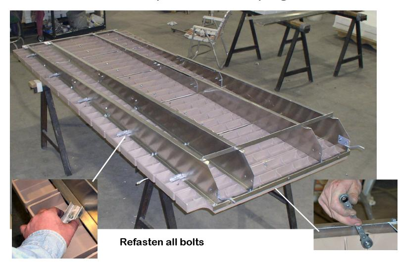
Drill four holes in ramp beams near where the 6' beam meets with the 10' beam. Fasten bottom brace with four 5/16 bolts and flange nuts
