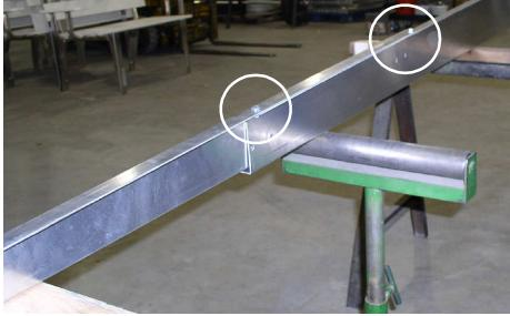
When frames are fastened you may need to drill holes on the side of the beams if the holes do not line up.
