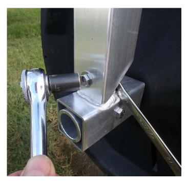
3. Remove the two bolts that connect the leg and tire to the axle. Leave the tire in place and swing the axle out of the way. This should free up the leg so you can shorten it.
