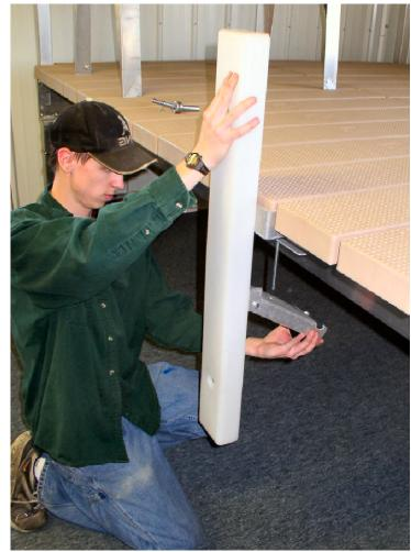
Next rotate bumper upright and swing the bottom arm so it grasps the bottom of the V-beam. Fasten carriage bolt & flange nut.
