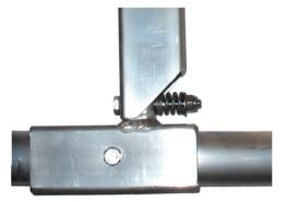
Note: tighten the lock nut so some of the threads just go beyond the lock nut ( leaving the spring flexable )
