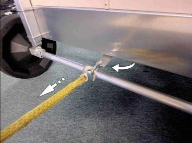
The quick hitch can swivel out so a tow rope can be attached as shown.
