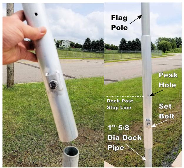
For the round Post attachment slide the attachment over an 1 5/8" round post. Loosen the set bolt, slide the round post brackets until you see the dock post in the peak hole.
