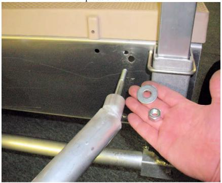
Secure with the washer and nut on the other side of the end channel as shown.
