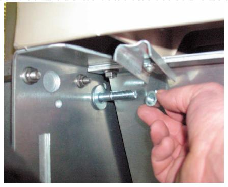
Note: Tongue can extend up to 10 feet or shorten it up if you prefer. Do this by removing and the bolt and nut, extending the tongue in or out, and then re-fasten the bolt.
