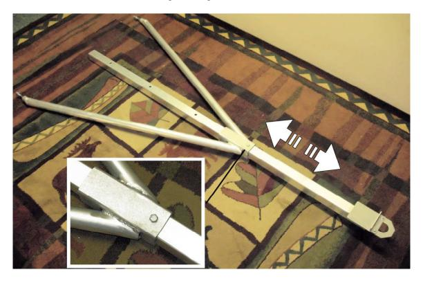
To lock the latch onto a ball, remove the one bolt with the flange nut. The other bolt, with the lock nut, will allow the latch to swing. After placing the tongue over the ball, resecure the latch with the bolt you removed and tighten the flange nut.
