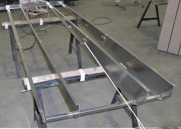
Fasten the remaing beams together. Align 4 beams as shown refasten bottom member and starter plate.
