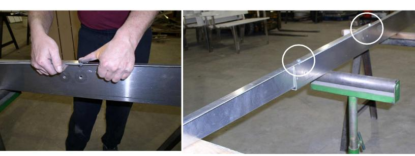
**Tightening guidelines** For 1/4" bolts and fasteners to 15- 20 foot-pounds For 5/16" bolts and fasteners to 20- 25 foot-pounds For 3/8" bolts and fasteners to 25- 30 foot-pounds
