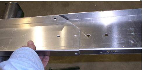
Connect the existing ramp beam to the 10' extension. Fasten with two 1/4 : bolts and flange nuts fasten on the top only.
