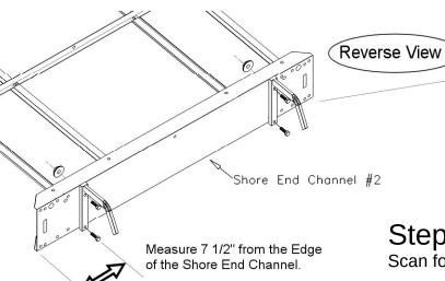
Measure 7 1/2" from the edge of the shore end channel and fasten hangers using (2) 5/16" x 1" hex head bolts and flange nuts as shown.
