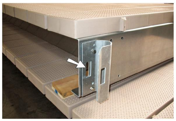
Place the post bracket on the end channel as shown. Make sure the square hole on the post bracket & the end channel are alligned. Fasten with (2) 5/16" x 3/4" hex head bolts & flange nuts
