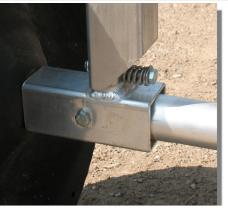
Slide the axle connection into the leg as shown. Tighten the spring bolt and lock nut until the theads of the bolt just goes beyond the lock nut leaving the spring flexable.
