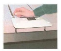
Step 3. Place cleat off the edge of the dock, next place (2) 1/4" x 3" hex head bolt & washers through cleat as shown Install cleat clip under decking and loosley hand tighten with a 1/4" flange nut.
