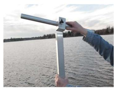
7. Slip the T-Handle onto the post and tighten in place. Tie the rope around the top of the T-Bar.
