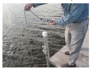
9. When the spiral anchor is at your desired depth, pull upward on the T-bar to release the anchor and pull the rope out of the water.
